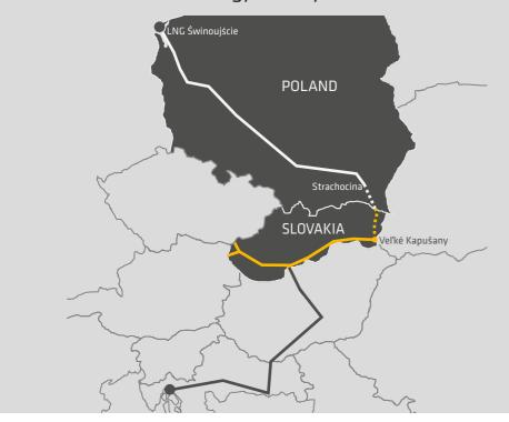
The Slovak part of the project includes the construction of a new bidirectional gas pipeline from the border with Poland at Lupkov Pass to the biggest compressor station in the European Union at Vel'ké Kapušany.
